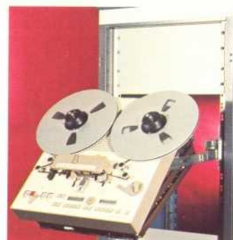
mounted on the 19" rack
