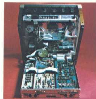
Hinge-mounted amplifier and tape transport electronics
